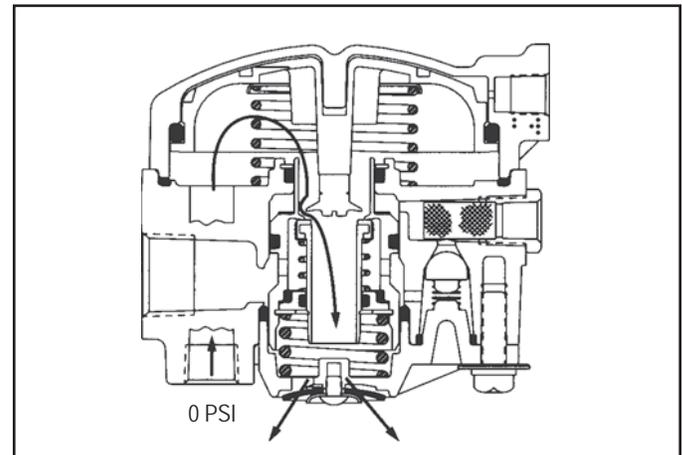
FIGURE 10 RE-6™ & RE-6NC™ RELAY VALVES SERVICE EXHAUST
