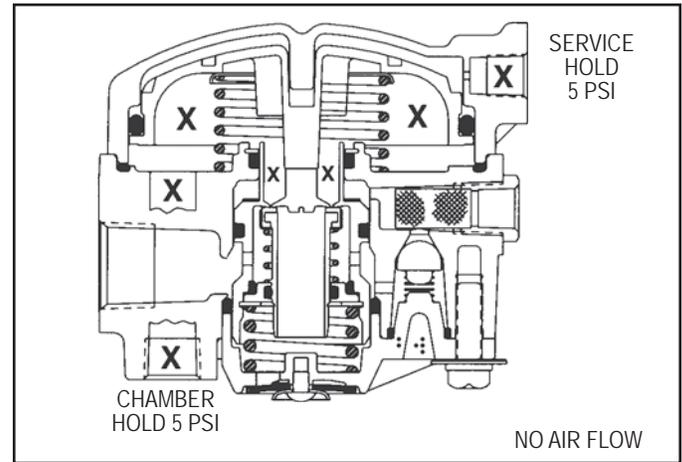
FIGURE 9 RE-6™ & RE-6NC™ RELAY VALVES SERVICE HOLD
