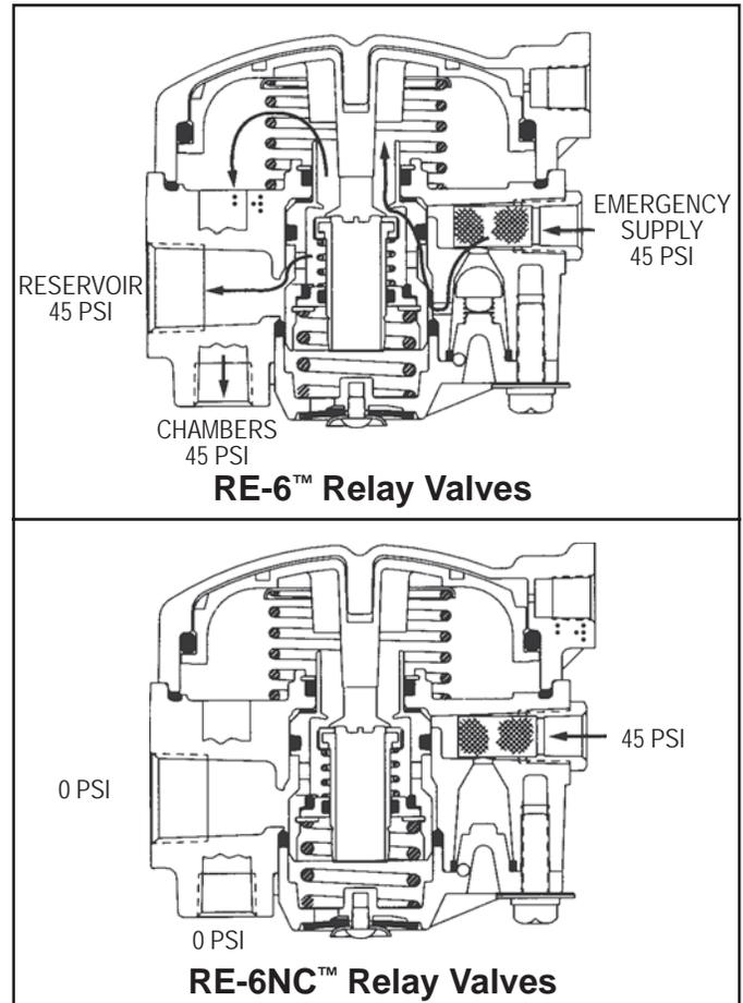
FIGURE 4 RE-6™ & RE-6NC™ RELAY VALVES CHARGING BELOW 45 PSI
