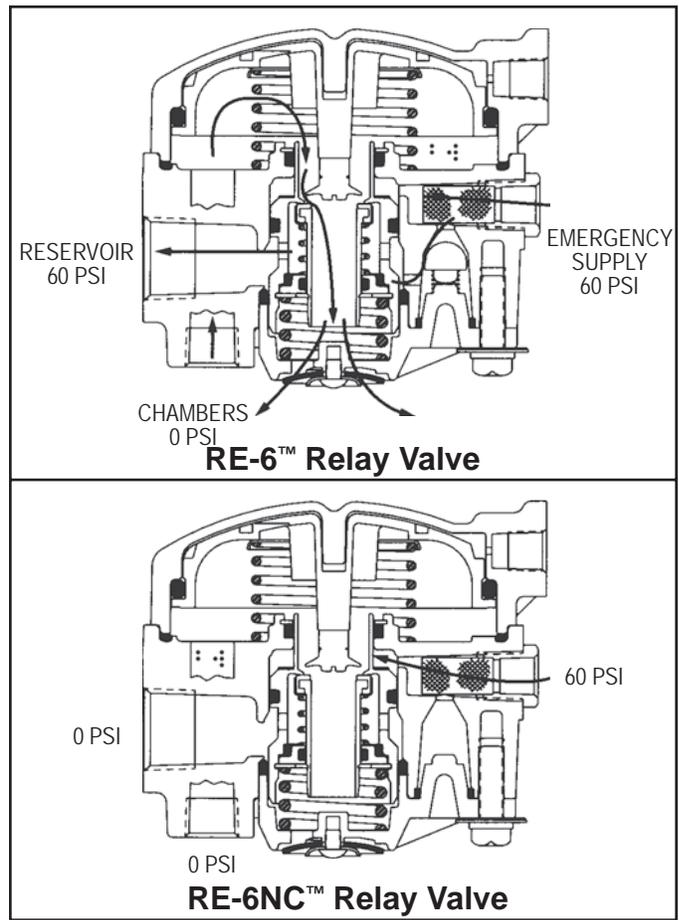
FIGURE 6 RE-6™ & RE-6NC™ RELAY VALVES CHARGING ABOVE 60 PSI
