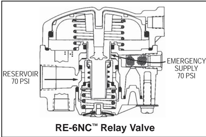
FIGURE 7 RE-6NC™ RELAY VALVE CHARGING ABOVE 70 PSI
