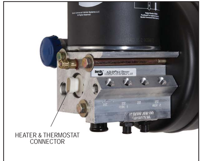
FIGURE 4 - HEATER AND THERMOSTAT CONNECTOR
