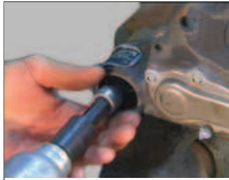
FIGURE 67 - REMOVE THE CALIPER BOLTS
