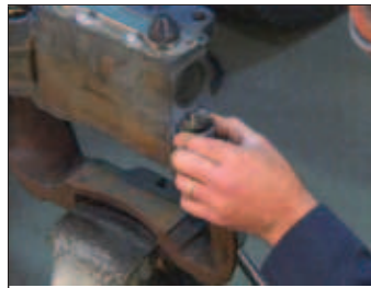
FIGURE 78 - POSITION THE NEW BUSHING
