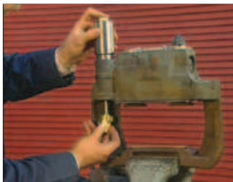
FIGURE 70 - INSTALL THE REMOVAL TOOL
