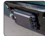
Bendix® FLR20™ Radar Sensor Mounted to the Vehicle Front
