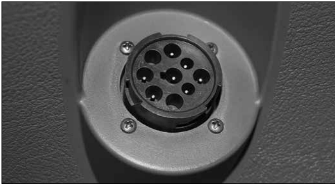
FIGURE 7 - TYPICAL VEHICLE DIAGNOSTIC CONNECTOR LOCATION (J1939)
