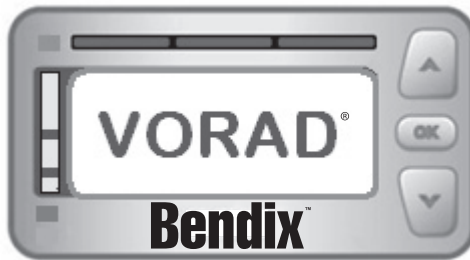
VS-400 DIU Lamp Test at initial power-up
