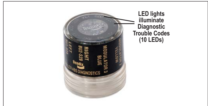
FIGURE 10 - THE BENDIX® TRAILER REMOTE DIAGNOSTIC UNIT (TRDU™)
